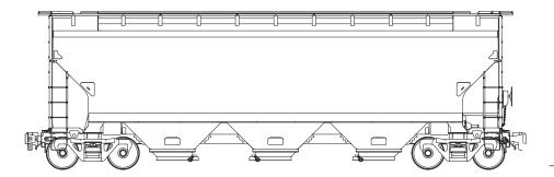
There are three different types of roof arrangements on the car: 1) Continuous trough (37' 6") (shown) 2) Segregated troughs (3 x 10' 4")
