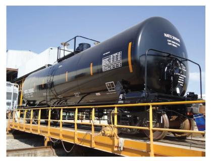
This 20,500 gallon tank car is designed for the transportation of Urea Ammonium Nitrate (non-regulated) and products authorized by DOT Part 173 for which there are no special commodity requirements and non-regulated commodities compatible with this class of car.
