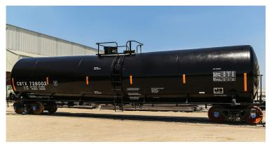
This 29,000 gallon (US) coiled and insulated tank car has been designed with a 286,000 lb gross rail load for the transportation of crude oil and other like commodities. The car is equipped with a 20-inch, eight (8) bolt manway, a 75 psi pressure relief valve, and a protected top fitting arrangement. Top fittings
