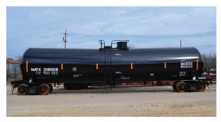
This 31,800 gallon (US) non-coiled and non-insulated tank car has been designed with a 286,000 lb gross rail load for the transportation of crude oil and other flammable liquids. The car is equipped with a 20-inch, eight (8) cast steel bolt style manway, and a 165 psi McKenzie pressure relief valve.
